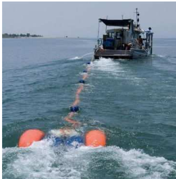
Figure 12. Acquisition using sparker source (@ Geo Marine Survey Systems)
