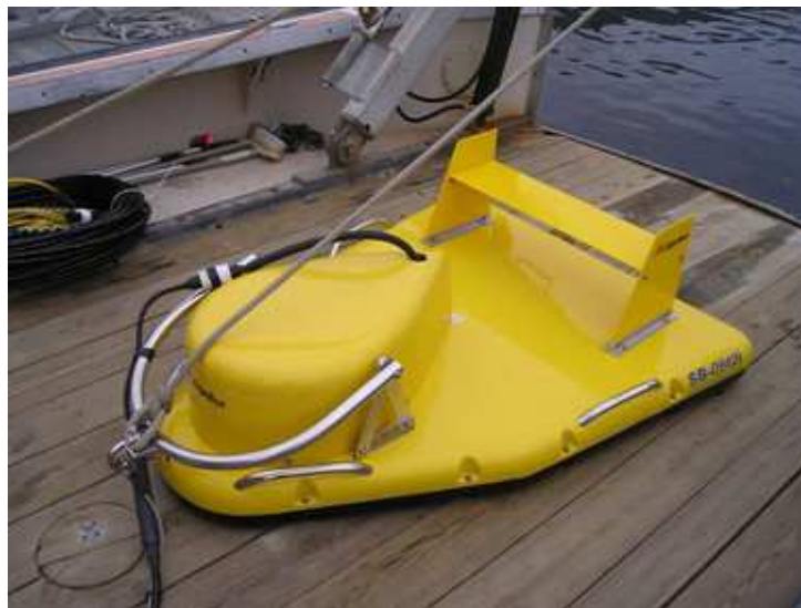
Figure 16. Typical Chirp towfish (© Edgetech)
