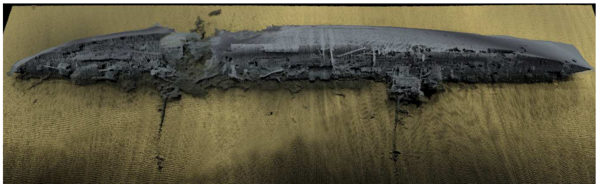
Figure 6. Multibeam Echosounder example on wrecksite From Adud Deepocean ( http://www.adus-uk.com/wreck-images )
