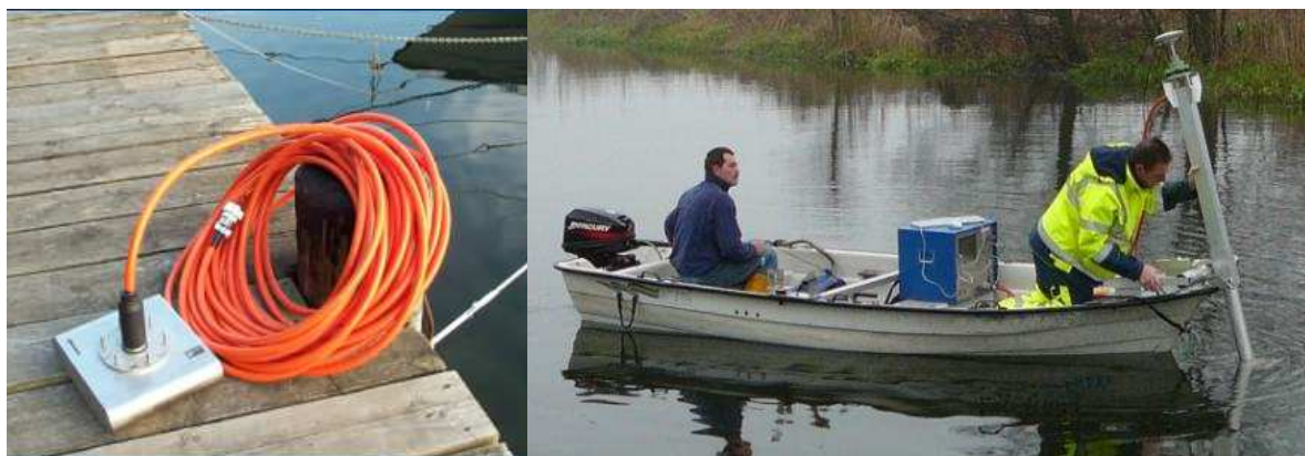
Figure 19. Parametric Echosounder transducer (left) and acquisition (right) (© Innomar)
